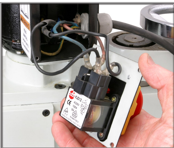
Figure 71. Mill power switch.
